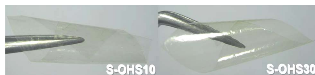
Fig. 3 Representative flexible and highly transparent PITE hybrid films (thickness: 15 \pm 3 \mu\text{m} ).
