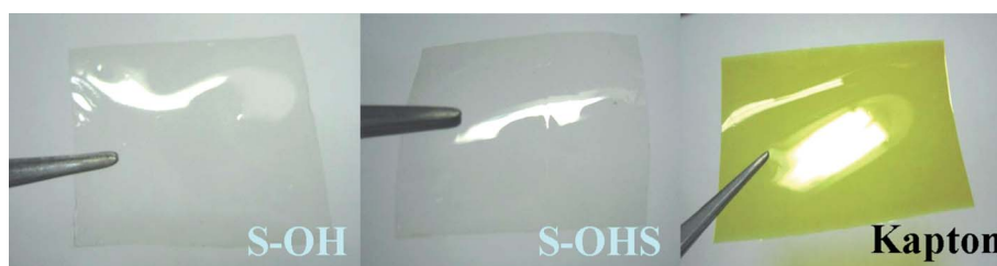
Fig. 2 Representative flexible and highly transparent PITE and Kapton films (thickness \sim 20 \mu\text{m} ).
